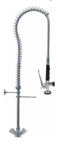
flow-rate spray gun 16l/min at 3 bar flow-rate swivel spout 32l/min at 3 bar
