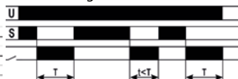
FZ76: ON delay with change-over contact
