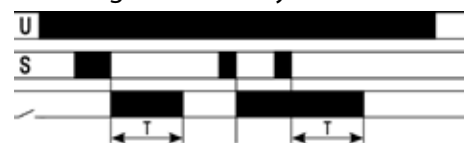
FZ81: Signal OFF delay
